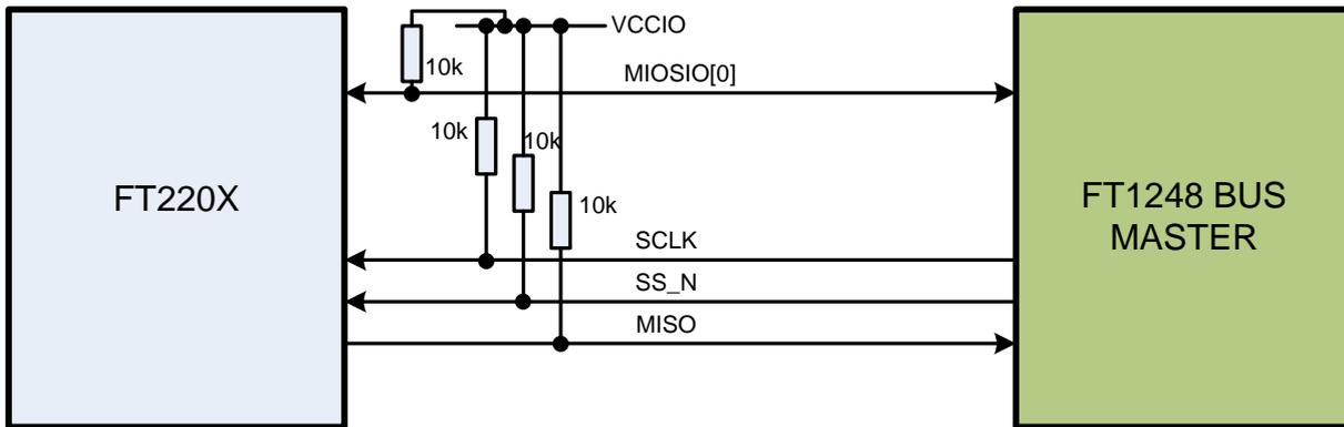
**Figure 8.1 Application Example showing USB to FT1248 host**
