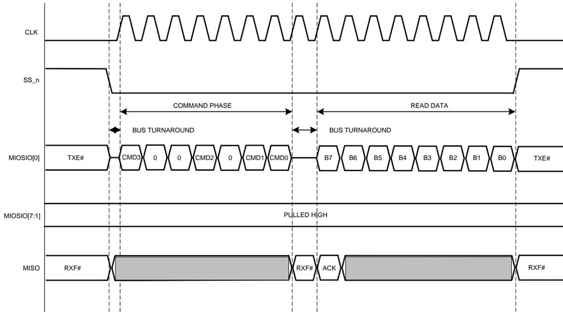
**Figure 8.3 FT1248 1- bit read timing diagram**
