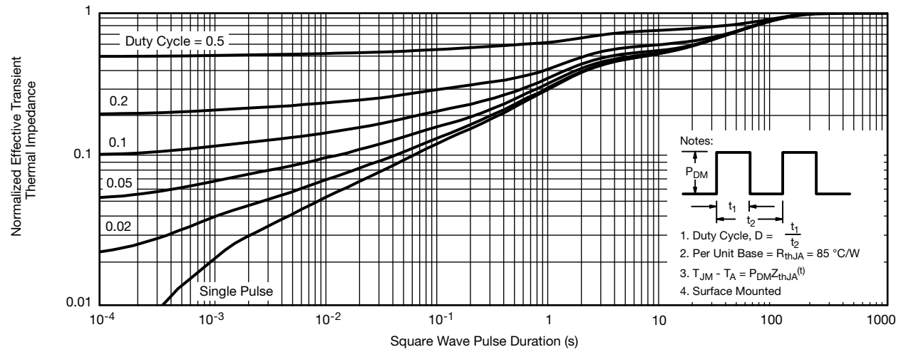
Normalized Thermal Transient Impedance, Junction-to-Ambient
