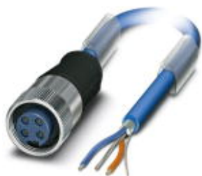
Sensor/actuator cable, FOUNDATION Fieldbus, 3-position, PVC, blue RAL 5015, free cable end, on Socket straight 7/8"-16UNF, A-coded, cable length: 15 m
