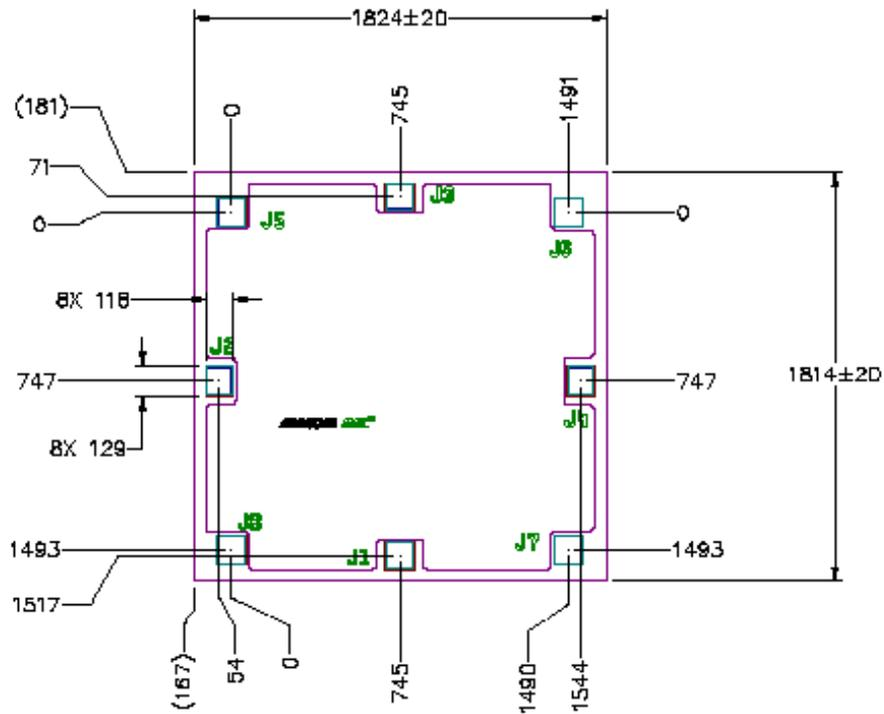
9. Unless otherwise specified, all dimensions shown as  $\mu\text{m}$ , with tolerance  $\pm 5 \mu\text{m}$ .
