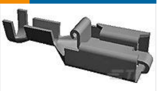
TE Part #880645-6 PL REC 1.0-2.5MM2 0.40 X 52.32 PTPBR
