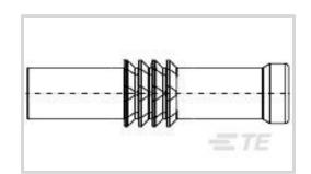
Connector Seal & Plug Type: Sealing Plug Primary Product Material: Silicone Rubber
