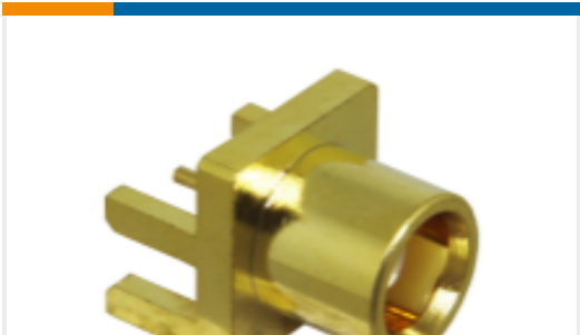
TE Part #L9000246-01 MCX Jack 50 Ohm .062 PCB Edge Mount
