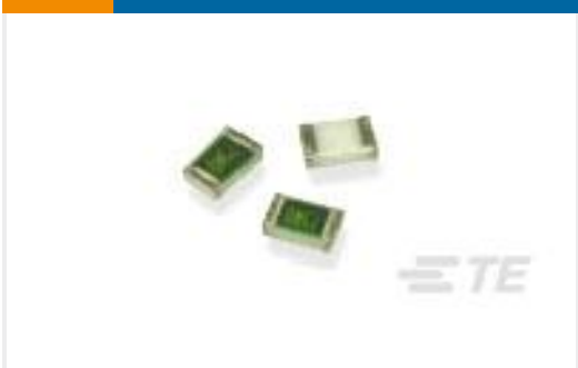
TE Part #3-1614354-4 RN 0603 61R9 0.1% 10PPM CUT LENGTH
