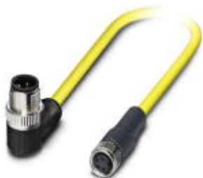
Sensor/actuator cable, 4-position, PVC, yellow, Plug angled M12 SPEEDCON, A-coded, on Socket straight M8, cable length: 1.5 m
