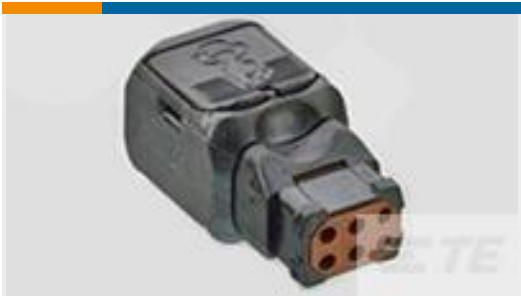
TE Part #D369-P66-NP1 369 6 WAY PLUG, CRIMP, PIN
