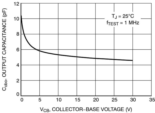
Figure 11. Output Capacitance
