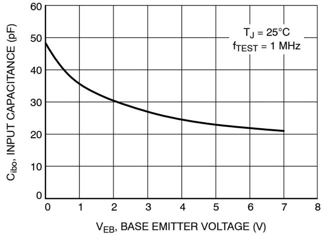
Figure 10. Input Capacitance
