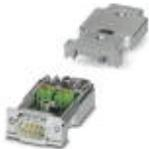
D-SUB connector, 9-pos., male connector, axial version with two cable entries, bus system: PROFIBUS DP up to 12 Mbps, termination resistor can be switched on via slide switch, pin assignment: 3, 5, 6, 8; spring-cage connection terminal blocks
