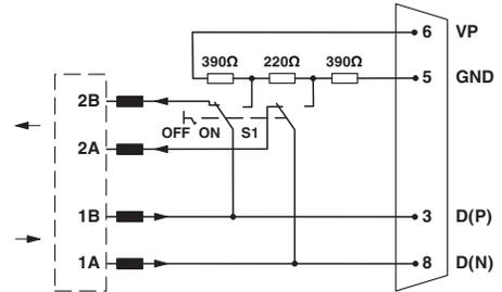
Functional diagram of the connector range
