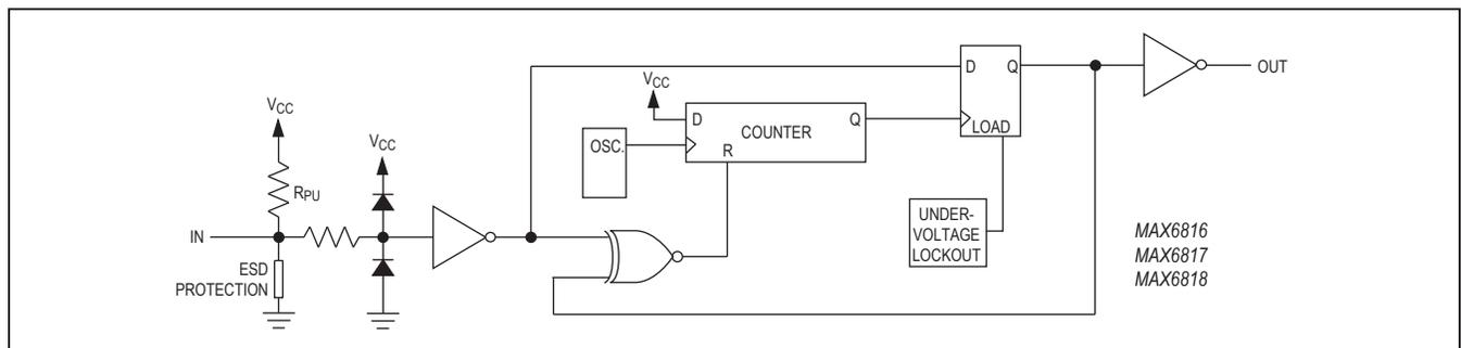
Figure 1. Block Diagram
