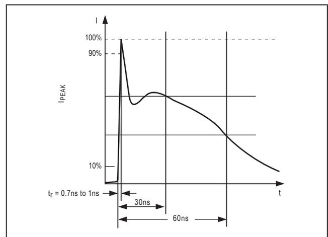
Figure 7b. IEC 1000-4-2 ESD Generator Current Waveform
