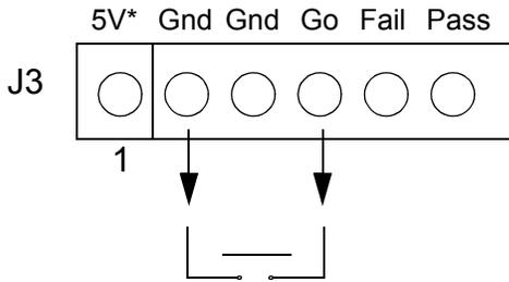
\*Not meant to power target. Reference voltage only (50 mA).
