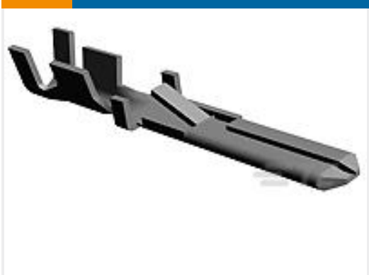
TE Part #928931-1 FF 110 (2.8 X 0.8 MM) TAB SSP CUZN30
