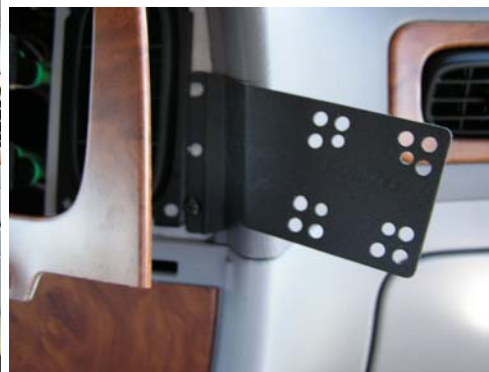
InDash fit into location with screw
