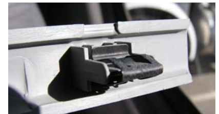
Clip to pull out slightly
