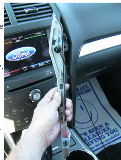
Bezel removal (plastic lug)
