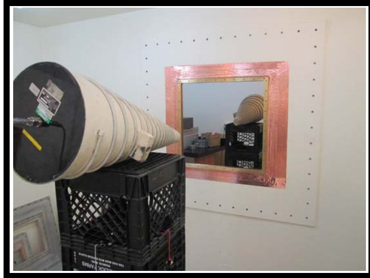
Open Reference Test Setup 200MHz to 1GHz
