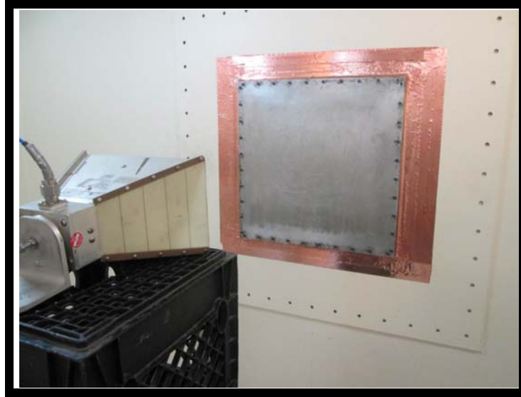
Closed Measurement Setup 1GHz to 10GHz
