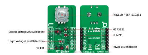
The output of the potentiometer is brought to the non-inverting input of the OPA344, a rail-torail operational amplifier from Texas Instruments, used as a stable unity gain buffer, providing a constant input and output impedance. Without a buffer, the variable impedance would affect the reference voltage. Therefore, the OPA344 ensures good stability of the circuit.
