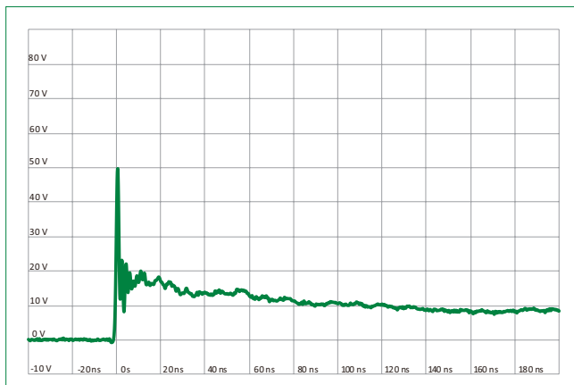
IEC 61000-4-2 +8 kV Contact ESD Clamping Voltage
