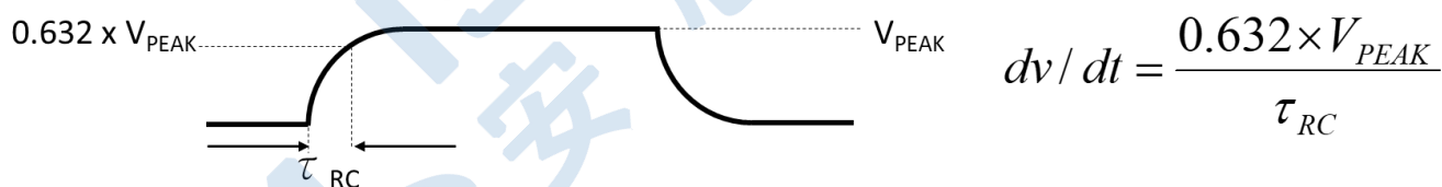
Fig.16 Waveforms of dV/dt
