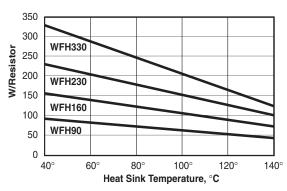
This graph shows the maximum wattage rating for each of the five possible ressistors of standard size corresponding to the heat sink temperature. It is assumed that all resistors are equally loaded. Please consult us about non-standard lengths and resistor modules.
