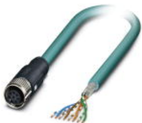
Assembled Ethernet cable, shielded, 4-pair, 26 AWG stranded (7-wire), RAL 5021 (water blue), M12 socket to free cable end, line, length: 25 m
