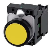
Pushbutton, 22 mm, round, plastic, yellow, pushbutton, flat, momentary contact type, with holder 1 NO, screw terminal, with laser labeling, inscription or symbol Customer-specific selection with SIRIUS ACT configurator (CIN)
