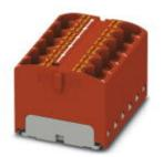
Distribution block, internally jumpered, nom. voltage: 630 V, nominal current: 32 A, connection method: Push-in connection, number of connections: 12, cross section:0.2 mm² - 6 mm², AWG: 24 - 10, width: 36.9 mm, height: 21.7 mm, color: red, mounting type: for snapping onto a DIN rail adapter, Adapter plate
