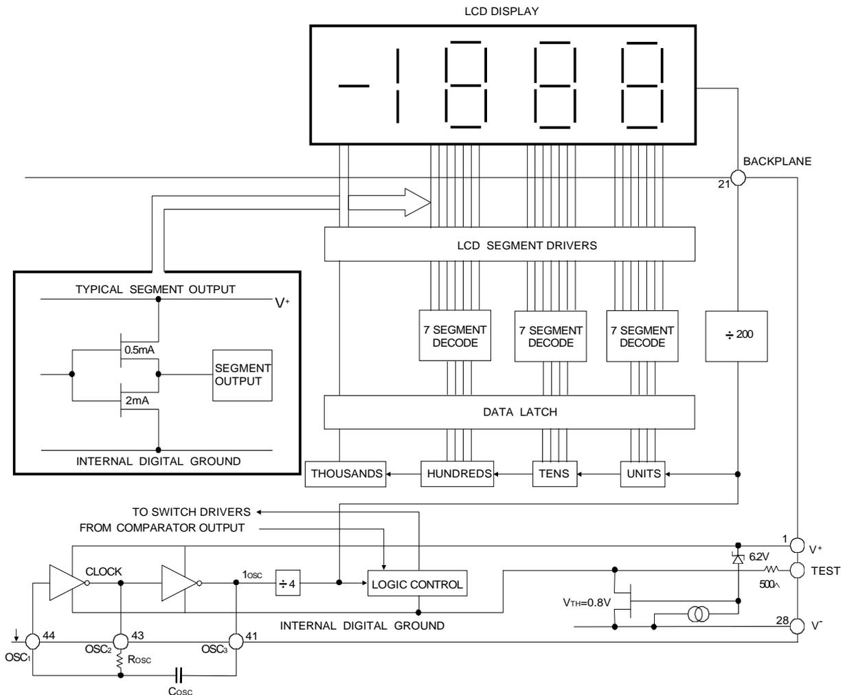
The internal digital ground is generated from a 6.2 volt Zener diode and a large p-channel follower. This supply is made stiff to adsorb the relatively large capacitive current when the back plane (BP) is switched. The BP frequency is the clock frequency divided by 800. The segments are driven at the same frequency and amplitude and are in phase with BP when OFF, but out of phase when ON. In all cases, negligible DC voltage exists across the segments.
