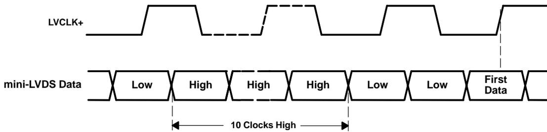
Figure 8. Reset Pulse Generation on mini-LVDS Data Pair
