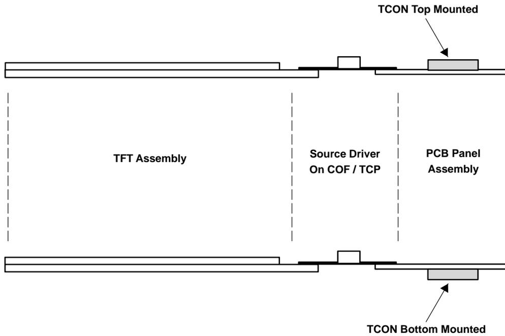
Figure 23. Definition of Top / Bottom Mounting
