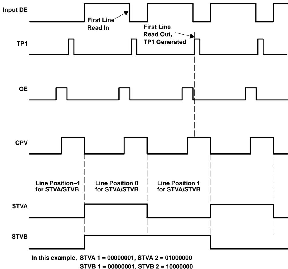
**Figure 2. Timing of Normal Operation**
