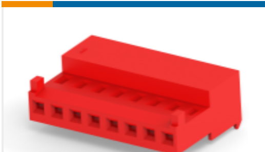
TE Part #3-644020-5 Nylon Gold Plated Receptacle: 2.54 mm, with Mating Alignment, MTA 100
