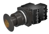
30mm BlackMax, Epoxy Coated Corrosion Resistant Complete Metal Unit Illuminated Push-Pull Operator Full Voltage, 24V AC/DC LED Lamp Mushroom Head Cap Small 1 3/4" (44.5 mm) Metal, Black with Amber Lens 3 Position Pull-Momentary/Push-Maintained 1 N.C.+1 N.C. Extra Late Break Heavy Duty Contacts, A600/P600 UL Listed, CSA Certified NEMA 1,3,3R,4,4X,12,13 & Automotive Standards
