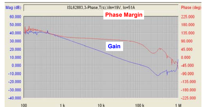
FIGURE 57. REFERENCE DESIGN LOOP GAIN T2(s) MEASUREMENT RESULT
