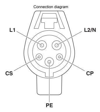
Pin assignment of the Vehicle Connector
