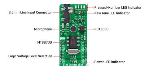
This Click board ™ has two ways to detect tones: with a mobile phone with a 3.5mm jack which provides the DTMF signals to MT8870D decoder, or using an onboard microphone used to listen the DTMF tones generated by the cell phone. The MT8870D uses digital counting techniques to detect and decode all 16 DTMF tone-pairs into a 4-bit code.
