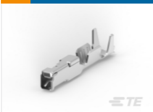
TE Part #2098762-3 Contact,female 0.64, 26 AWG, CuNiSi, Sn
