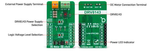
The device operates from a single power supply input (VM) available on the output terminal. The DC Motor 27 Click offers a VM SEL jumper that allows you to choose the power supply input from the external over the VEXT terminal and a 5V from the power rail of the mikroBUS™ socket. The EXT is set by default, so you should apply the appropriate voltage on the VEXT terminal.
