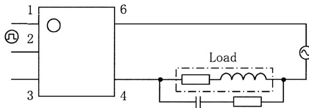
CR Snubber is connected in parallel with the load
