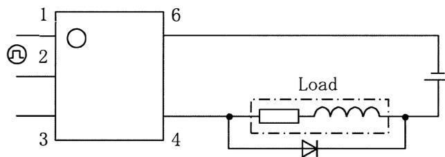
Clamp diode is connected in parallel with the load
