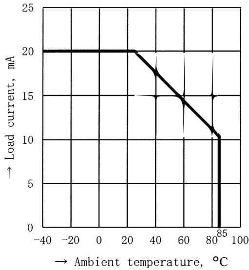
6- 2 LED forward current vs. Ambient temperature characteristics
