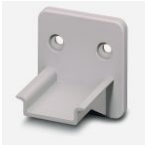
Plastic mounting bracket, with NS 35/7.5 DIN rail, to snap onto modular terminal blocks with a universal foot, profile length: 35 mm
