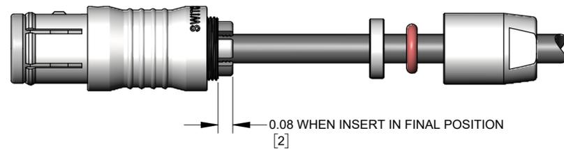
ALIGN INSERT ASSEMBLY INTO SHELL FOLLOWED BY THE CLAMP. PUSH CLAMP LIGHTLY FORWARD AND ROTATE UNTIL THE ASSEMBLY SNAPS IN THE FINAL POSITION SHOWN.
