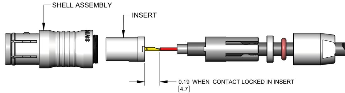
GUIDE EACH WIRED CONTACT INTO INSERT HOLE AND PUSH UNTIL CONTACT SNAPS IN PLACE. USE INSERTION TOOL\* IF NECESSARY.
