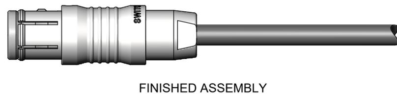
SLIDE WASHER, O-RING, AND NUT AGAINST CLAMP AND THREAD NUT ON UNTIL TIGHT - NOT TO EXCEED 9 IN-LB [1 Nm] TORQUE. A 5/16" [8 mm] WRENCH CAN BE USED, IF NECESSARY.
