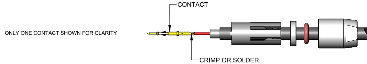
CRIMP CONDUCTORS TO CONTACTS USING HAND OR PNEUMATIC CRIMP TOOL\* WITH CRIMP POSITIONER\* SET PER CONTACT SIZE AND WIRE GAGE.
