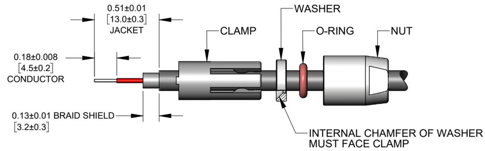
FEED THE FREE END OF CABLE THROUGH THE NUT, O-RING, WASHER, AND CLAMP IN THE ORDER SHOWN.
