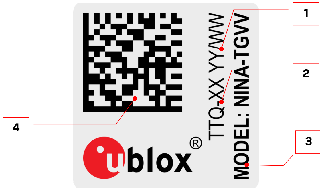
Figure 13: Location of product type number on the NINA-B4 series module label
