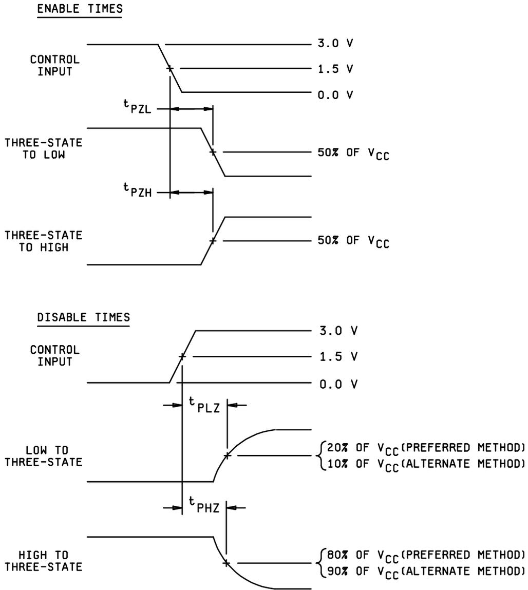
FIGURE 4. Switching waveforms and test circuit – Continued.
