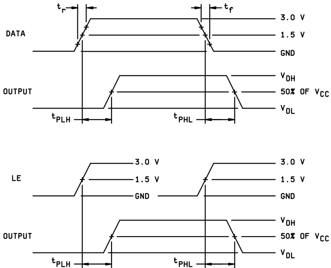
FIGURE 4. Switching waveforms and test circuit.
