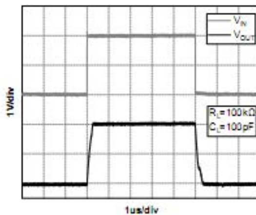
Figure 7. Large-Signal Step Response( V_S=5\text{V} )
