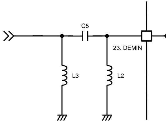
Figure 19. Equivalent Circuit for MIXER Input Block
