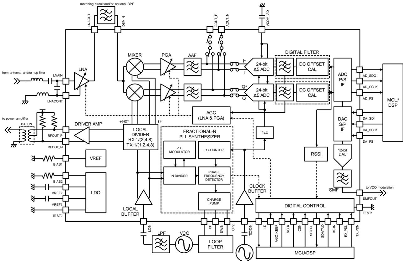
Figure 1. AK2401A Block Diagram
