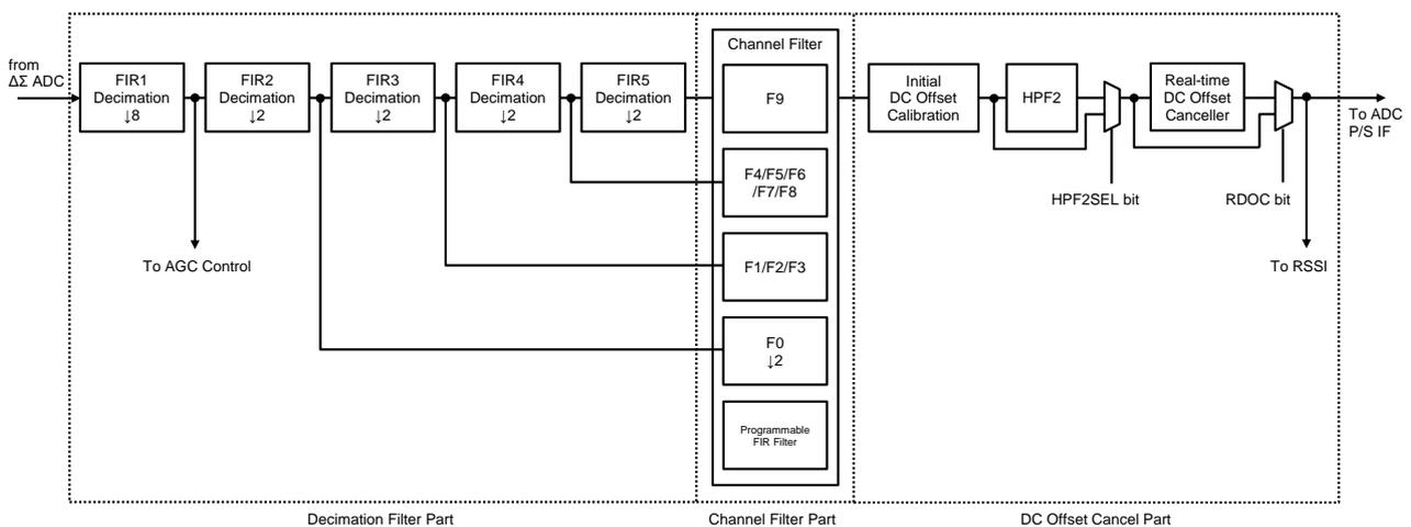
Figure 28. Digital Receiving Circuit
