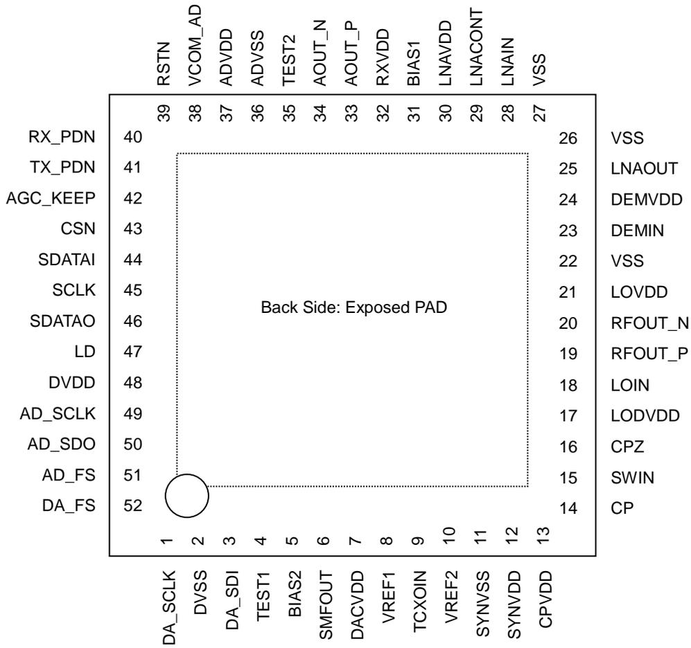
Figure 2. Pin Configurations (52-pin QFN0707, Top View)
