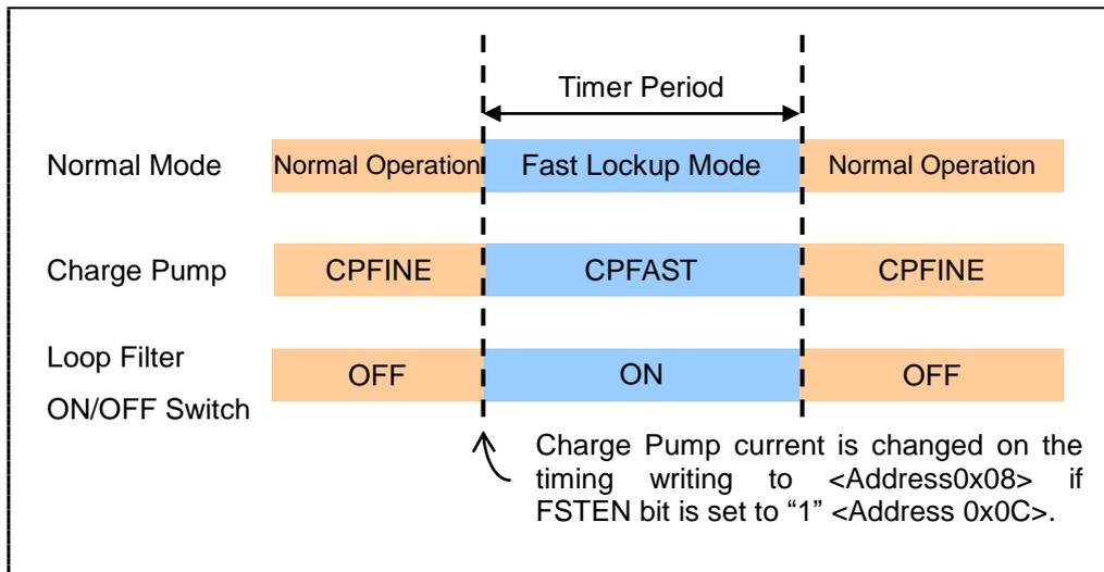
Figure 25. Fast Lock Function Sequence
