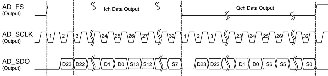
Figure 7. Interface Timing for ADC Data Read
