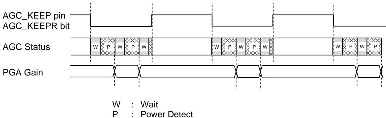
Figure 38. AGC Operation when AGCKP\_MODE[1:0] bits= “00”
