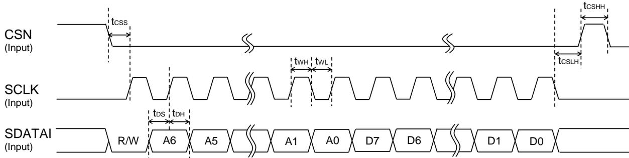
Figure 4. Interface Timing for Serial Register Write
