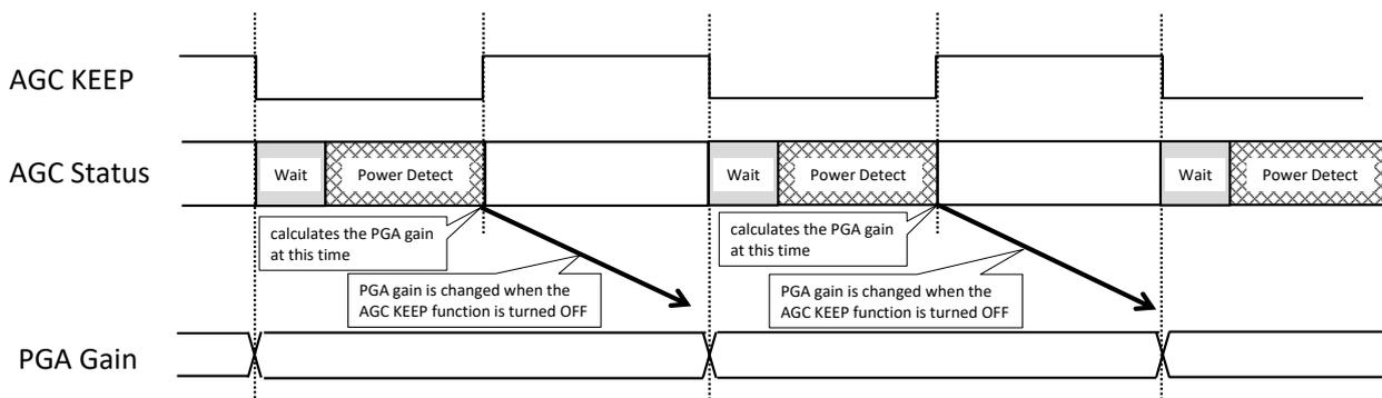
Figure 39. AGC Operation when AGCKP\_MODE[1:0] bit= “01”
