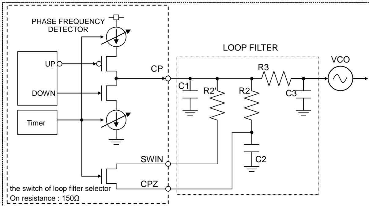
Figure 23. Charge Pump and External Loop Filter Circuit Example
