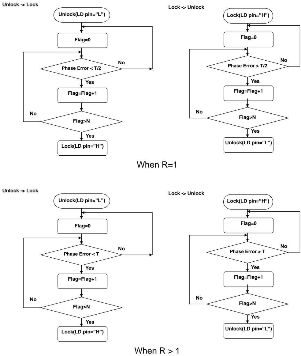
Figure 27. Flow Chart of PLL Lock Detection Function
