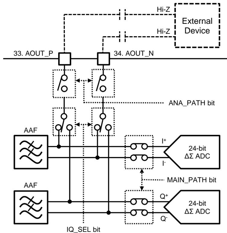
Figure 21. Output Path Selection of Analog Baseband Signal
