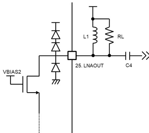
Figure 17. Equivalent Circuit for LNA Output Block
