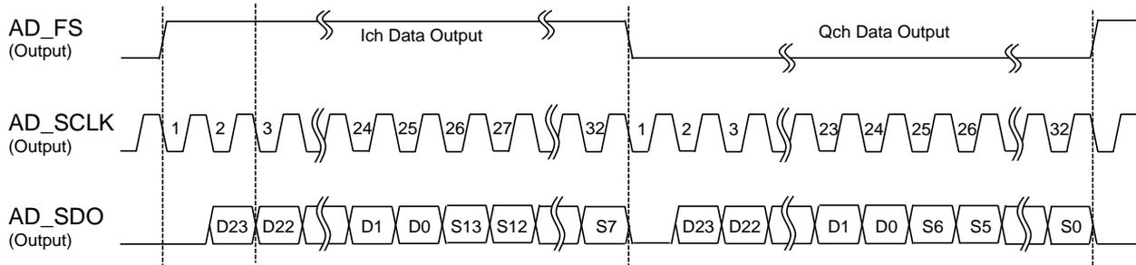
Figure 42. ADC Output Serial Interface Timing (Status Read)
