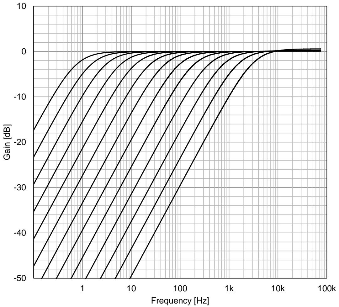
Figure 34. High-Pass Filter Frequency Characteristics
