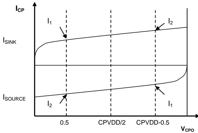
Figure 9. Charge Pump Characteristics - Voltage vs. Current
