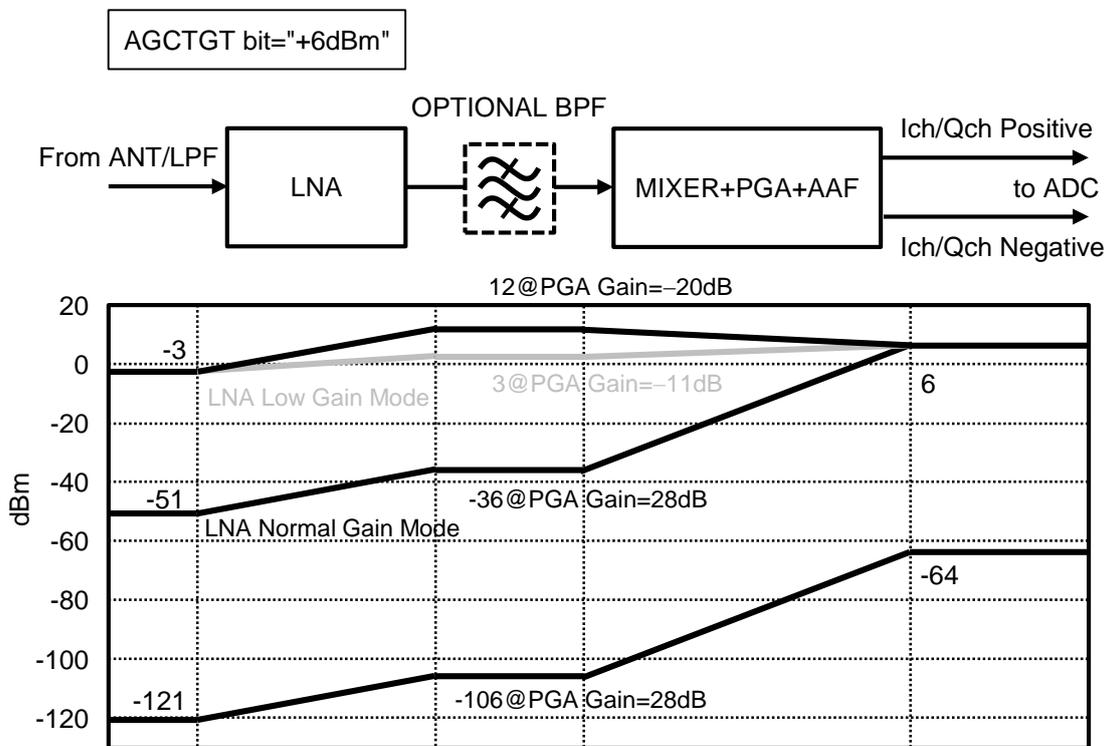
Figure 14. Level Diagram of Analog Receiving Circuit
