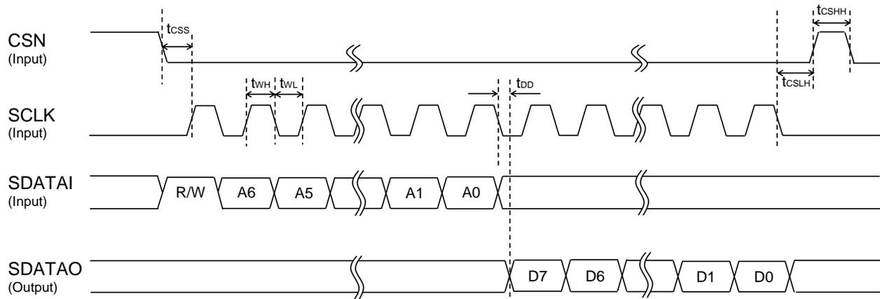
Figure 5. Interface Timing for Serial Register Read
