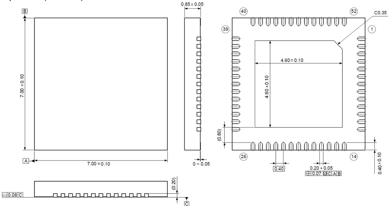
\*The exposed pad on the bottom surface of the package must be connected to VSS.
