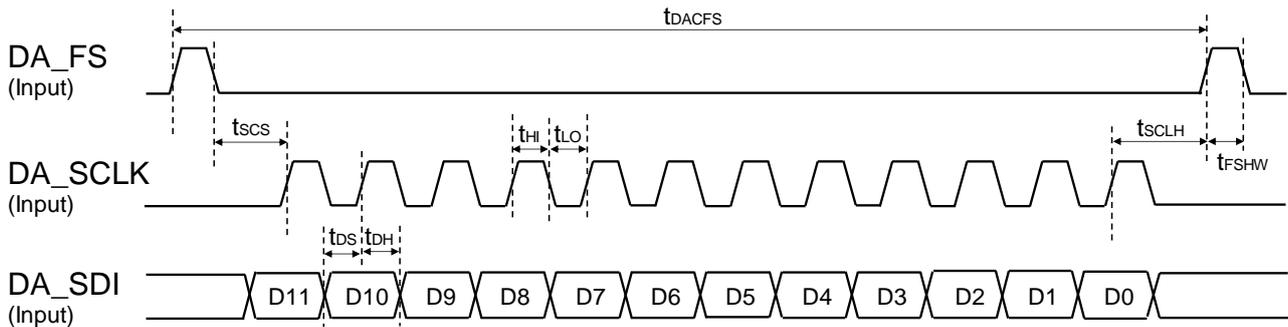
Figure 8. Interface Timing for DAC Data Write
