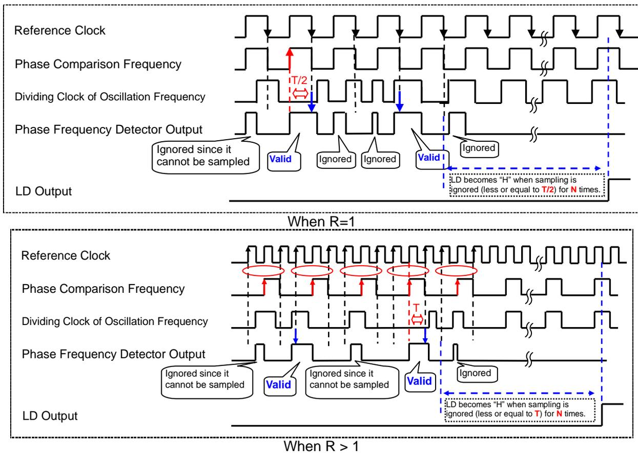
Figure 26 Digital Lock Detect Operations
