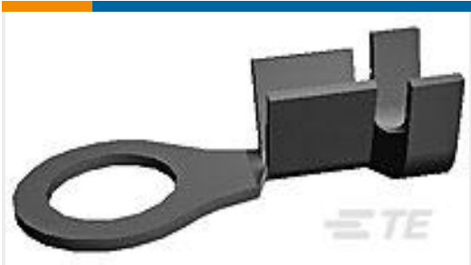
TE Part #880626-2 RING TONGUE 0.5-1.0 MM2 0.60X13.23 TPBR
