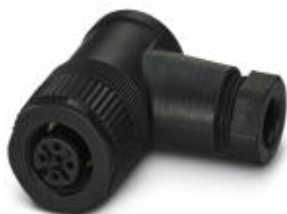
Connector, Universal, 5-position, Socket angled M12, A-coded, Screw connection, knurl material: Plastic, cable gland Pg7, external cable diameter 4 mm ... 6 mm
