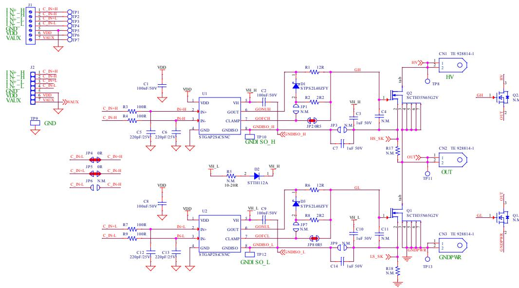
Figure 2. EVSTGAP2SiCSNC circuit schematic – supply, connectors and decoupling
