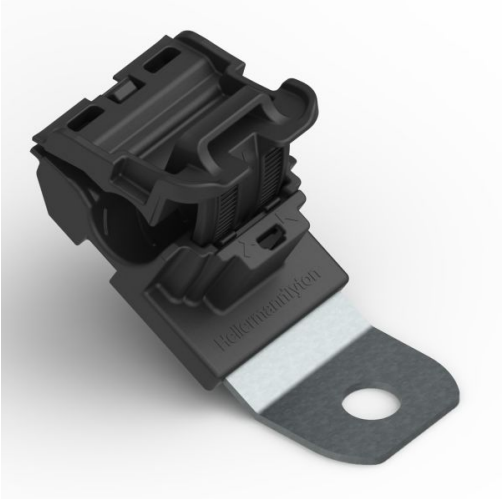
Ratchet P-Clamp, 0.24 - 0.54" Bundle Dia, 30° Long, .33" Hole Dia, PA66HIRHSUV/SS304, Black, 200/ctn
