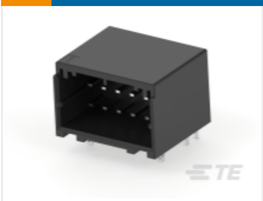
TE Part #1-1871468-2 Header Assembly: Wire-to-Board, 5A, gold or tin plated
