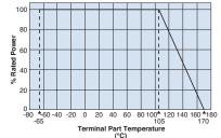
For resistors operated at a terminal part temperature of described for each size or above, a power rating shall be derated in accordance with the derating curve.
