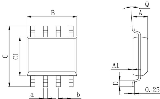
**Dimensions In Millimeters(SOP8)**
