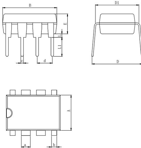
**Dimensions In Millimeters(DIP8)**
