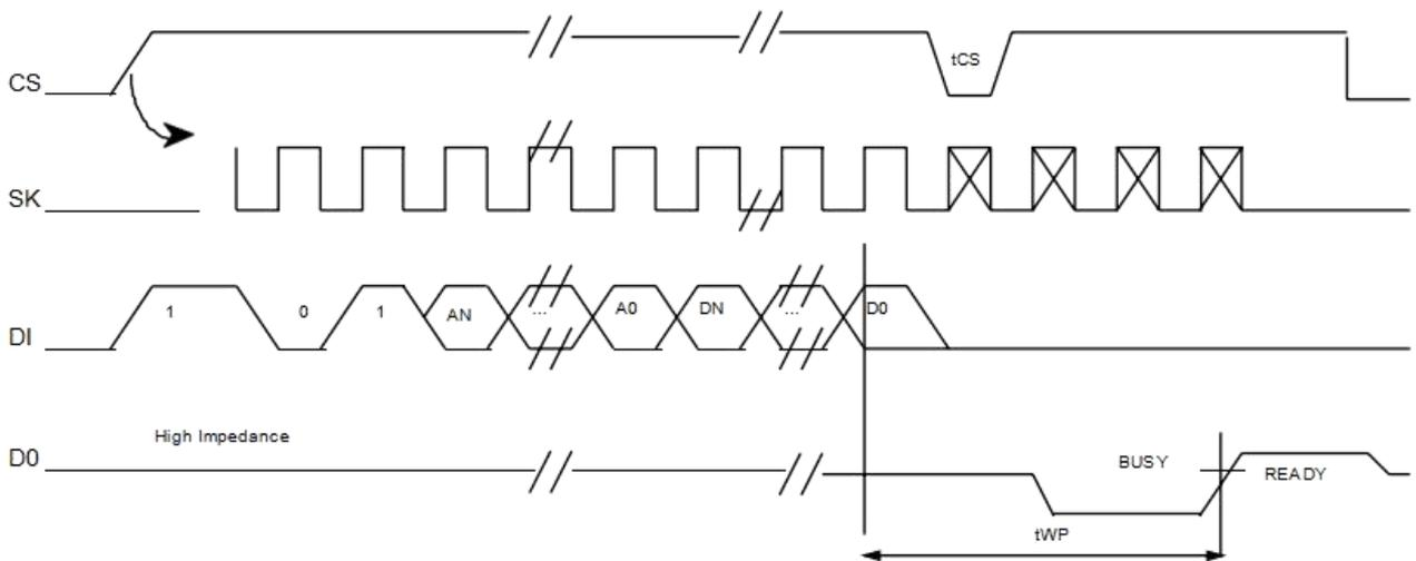
(1) Valid only at  $V_{cc} = 4.5V$  to  $5.5V$
