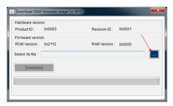
Click on the "..." and select the "Bosch\_PCB\_7183\_di01\_BMA2x2\_BMM150-7183\_di01.2.1.xxxxx" located in the "C:\Program Files\Bosch Sensortec\Development Desktop 2.0\Firmware\BHA" folder on your computer.
