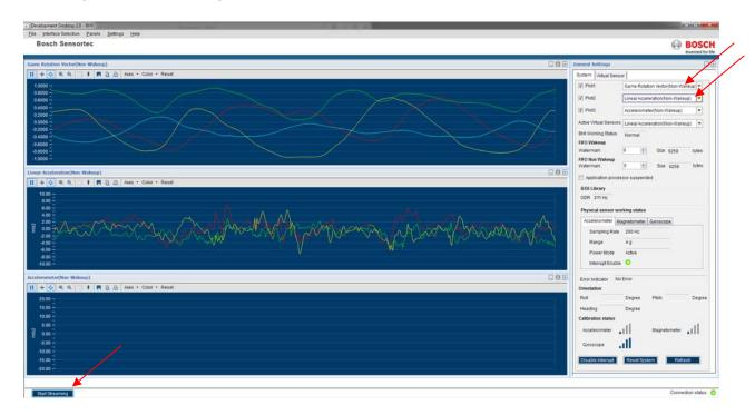
You should now see quaternion data with 50Hz Output data rate, Linear acceleration with 100Hz Output data rate, both at 100Hz Refresh rate.
