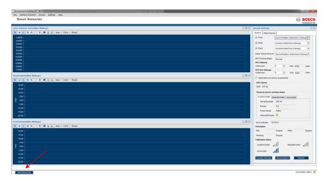
You should now see quaternion data with 50Hz Output data rate, 4Hz Refresh rate (1/250ms = 4Hz).
