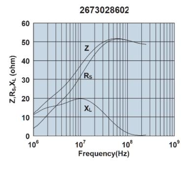
Impedance, reactance, and resistance vs. frequency.
